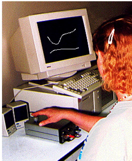
Figure 37: The Sentograph (Clynes, 1978). A two-dimensional touch transducer for biocybernetic measurements of finger pressure.
